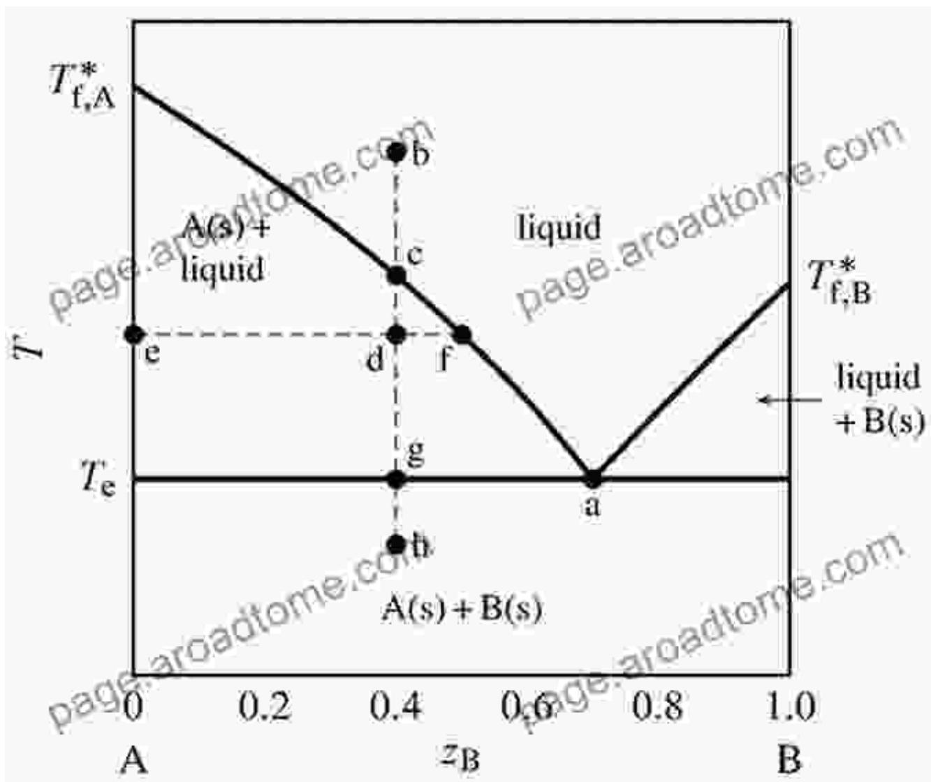
A phase diagram of a binary mixture, showcasing the different phases that coexist at various temperatures and compositions.
